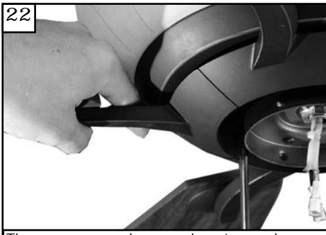
22 The screws, washers and motor pads are pre-installed to the blade holders. Attach blade assembly to motor and tighten screws securely.
